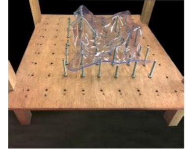
Figure 6, Resultant form after sheet being subjected to heat
